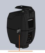
The microSD card is inserted on the slot on the side of the robot.
