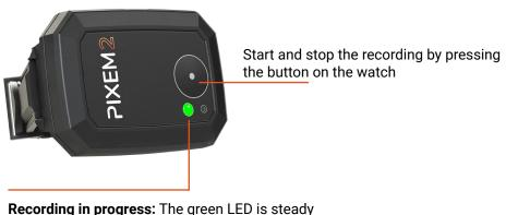
Recording in progress: The green LED is steady Recording stopped: The green LED is blinking
